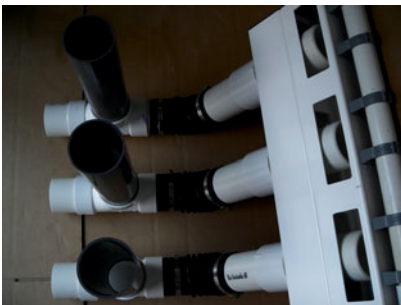
This multiple outlet Flout can dose three disposal area sections or combine to achieve a larger flow rate
