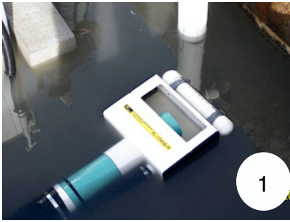
1. The Flout® is free floating, hinging on the flexible connector as the chamber fills. 2 When the Flout reaches maximum, liquid spills in, sinking it and opening the outlet to flow. 3. As the liquid drains down to the top of the Flout, it empties and begins to float again, closing the outlet
