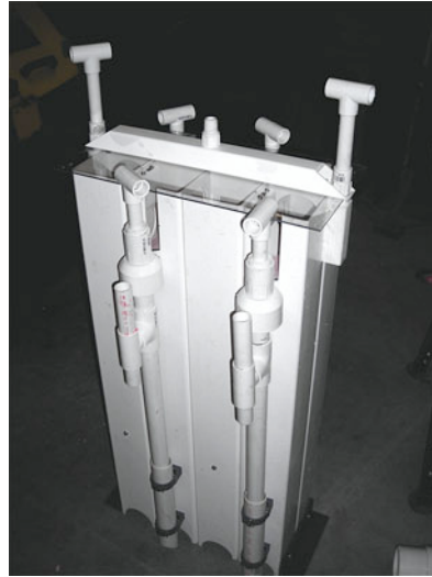
A CueBox™ for sequencing four 28 inch drawdown Flouts.
